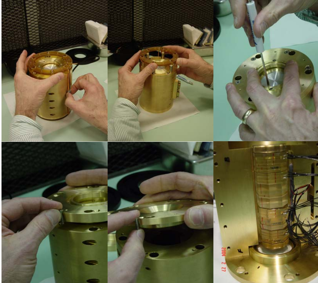
Figure 6. Disassembly of the filter.
