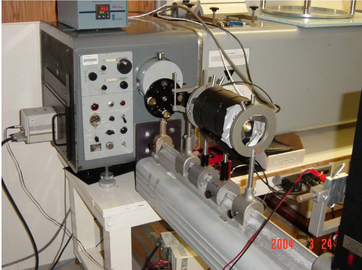
Figure 8. Filter optical test setup.
